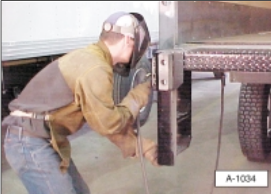
Illustration 17b. Tack weld dock bumpers.
