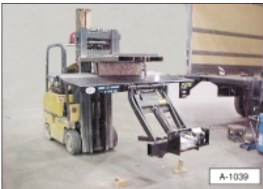
Illustration 5a. Use a forklift or overhead crane to lift the liftgate.
