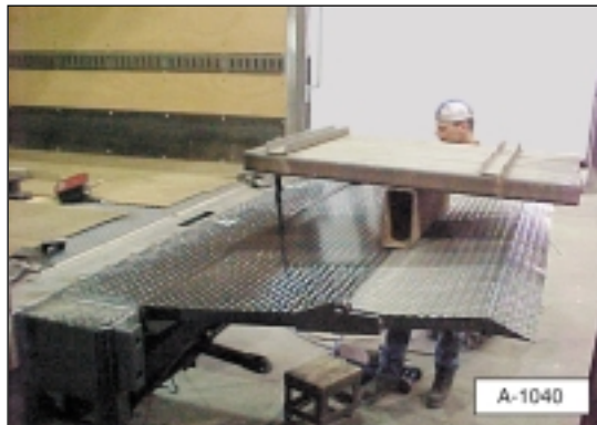
Illustration 5b. Align the center mark of the liftgate platform with the center mark on the floor extension.
