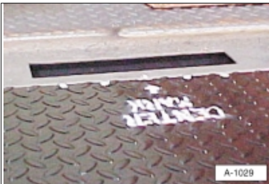
Illustration 4a. Align floor extension with mark.
