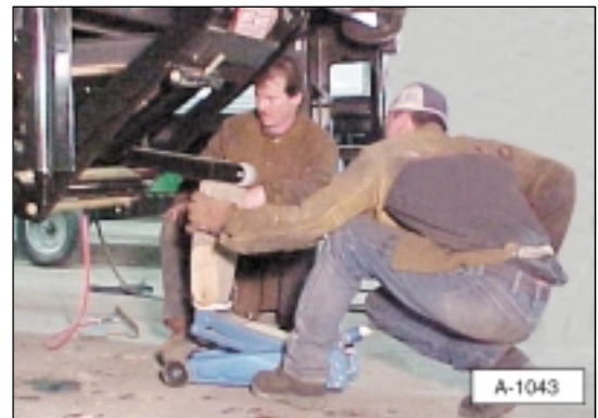
Illustration 8. Raise the tube assembly into place.
