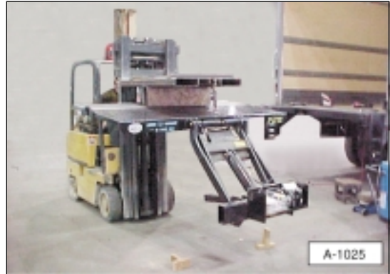
Lifting jig attached to liftgate. Lifting jig must support liftgate in a level position, as shown.
