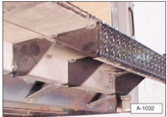
Illustration 4c. Tack weld floor extension brackets.
