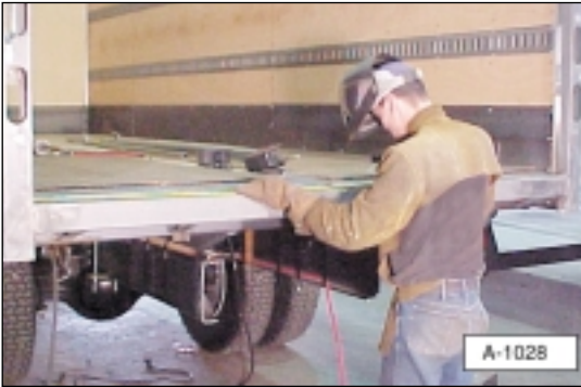
Illustration 3. Find and mark the center of truck's rear sill.
