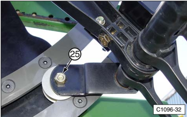
(24) Ball Bearing Roller. (25) Locknut.
